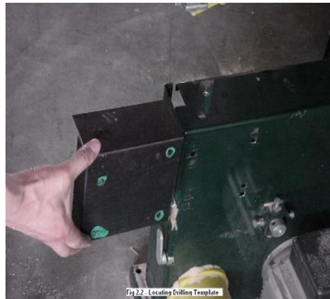
Fig 2.2 - Locating Drilling Template
